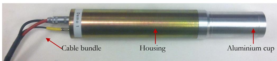
Figure 3-1. The components of the ISIS Neutron Beam Monitor.
