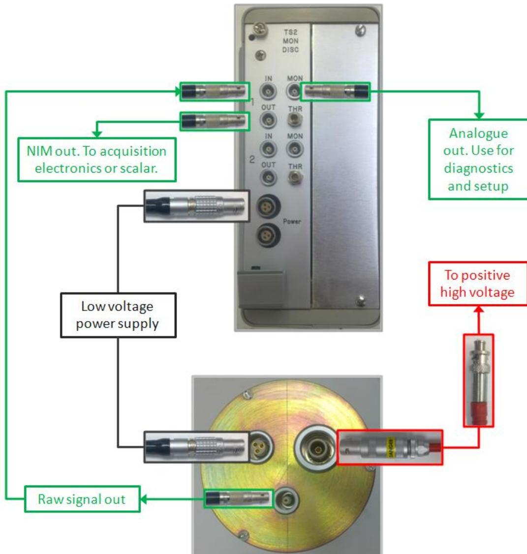
**Figure 4-2. Wiring diagram for the ISIS beam monitor. GREEN indicates signal cables (LEMO size 00.) BLACK indicates the 3-pin low voltage power supply. RED indicates the high voltage power supply. Please, note that a high voltage supply unit has not been shipped.**
