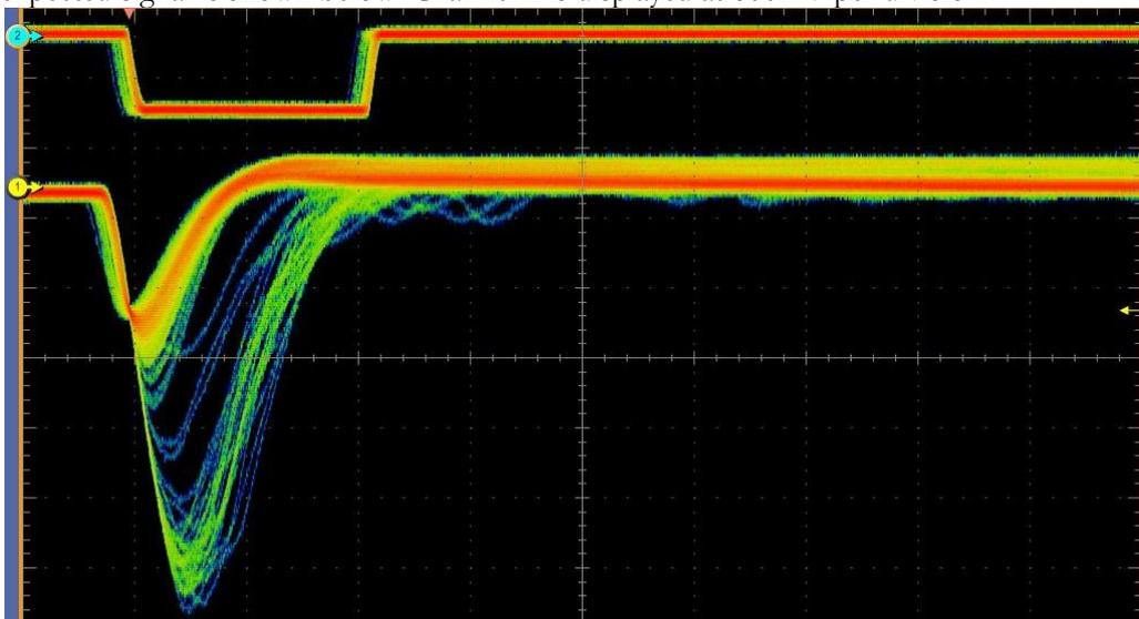
Adjust the scope to trigger on the digital output signal at about -600mV. This is shown as channel 2 below. Channel 1 will now only display pulses that are being counted as neutrons by the discriminator electronics. Often the threshold is too low, and tube noise and gamma events are being counted as well as neutron
