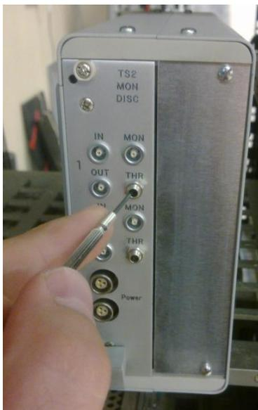
Figure 5-2. Adjusting the discrimination threshold using a small flat-head screwdriver.
