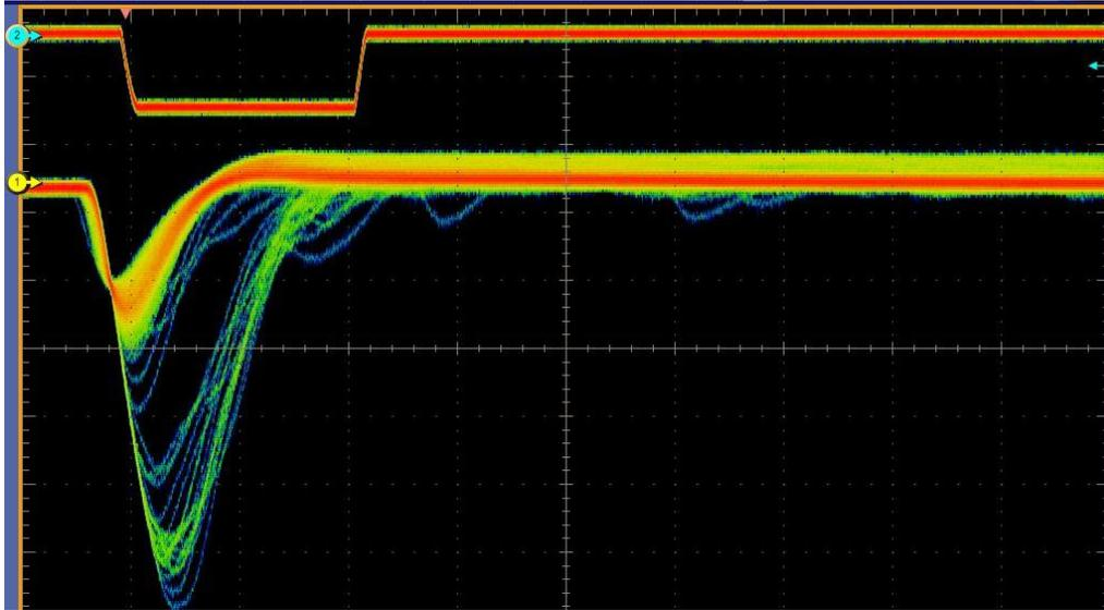
The pot should now be adjusted so that the only signals being displayed on channel 1 are neutron signals. In the above oscilloscope screen shot this would be a level of about -700mv. A larger negative discrimination is achieved by rotating the pot clockwise. The plot below shows the discrimination threshold set to the appropriate level.
