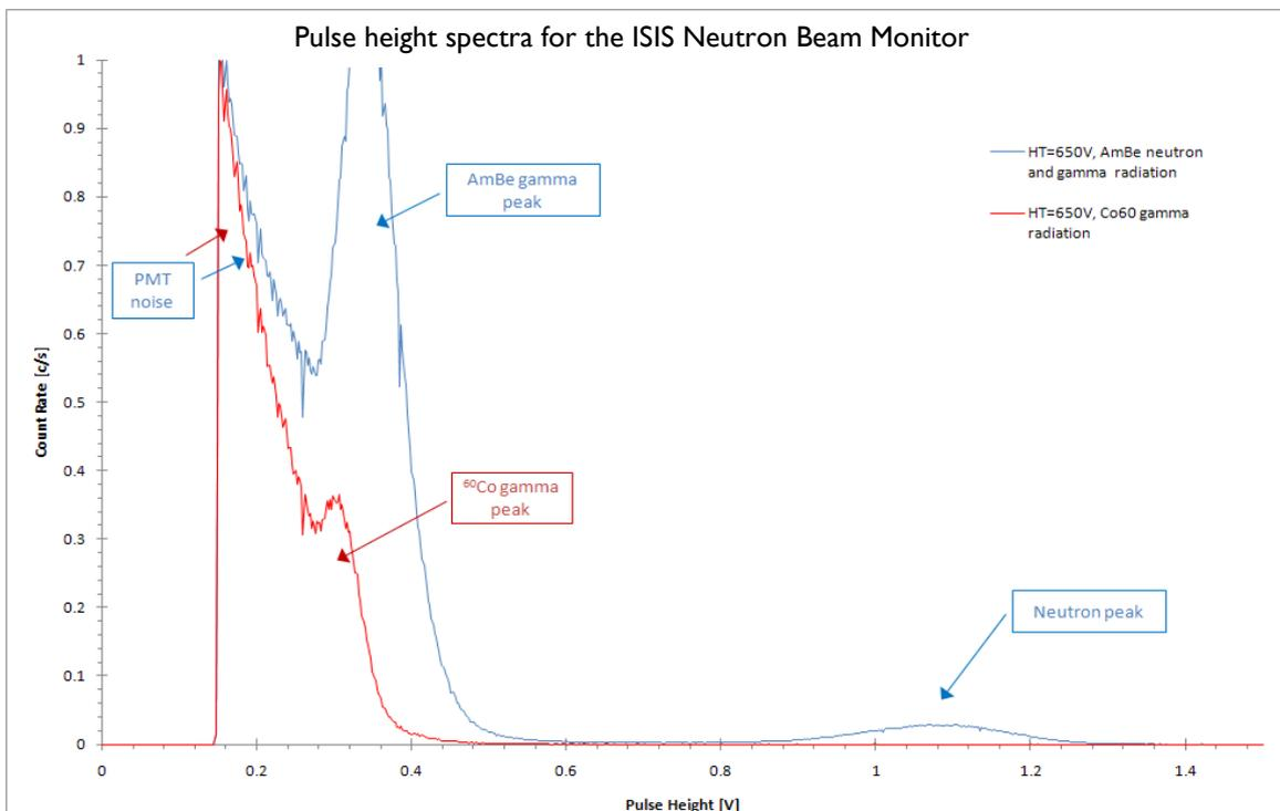
Figure 3-3. Pulse height spectra for the Neutron Beam Monitor DEMO I. This is the full data set, showing tube noise and gamma peaks. This is the same data used to produce Figure 3-2.
