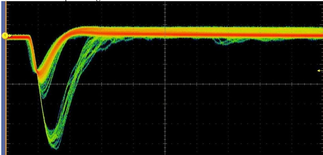
Display the digital out on channel 2 on the oscilloscope, while still triggering on channel 1. If a digital pulse does not appear lower the discrimination threshold. This is done using a small screwdriver, rotating anticlockwise. Rotate the pot until the digital pulses are at least as frequent as the neutron events. The expected signal is shown below. Channel 2 is displayed at 800mV per division.
