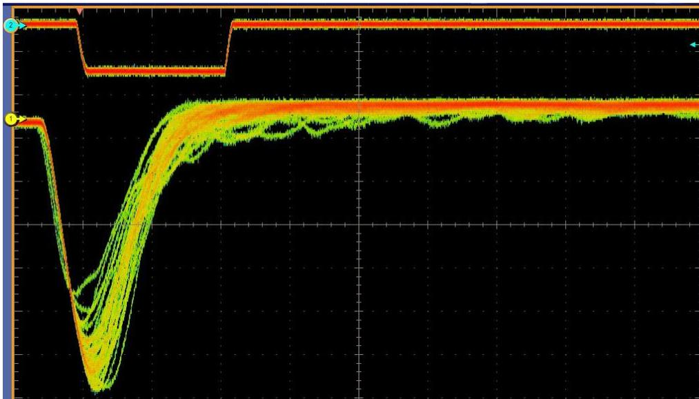
It is important to keep in mind the pulse height distribution for gamma and neutron radiation. By adjusting the pot the discrimination threshold has moved into the valley seen in the blue data set, shown in Figure 3-2. A discrimination threshold of -700mV is appropriate here as it ensures that all neutron events are counted, with minimal gamma events being included.
