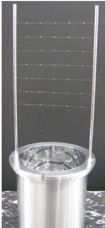
Figure I-1. The ISIS Neutron Beam Monitor scintillator array.
