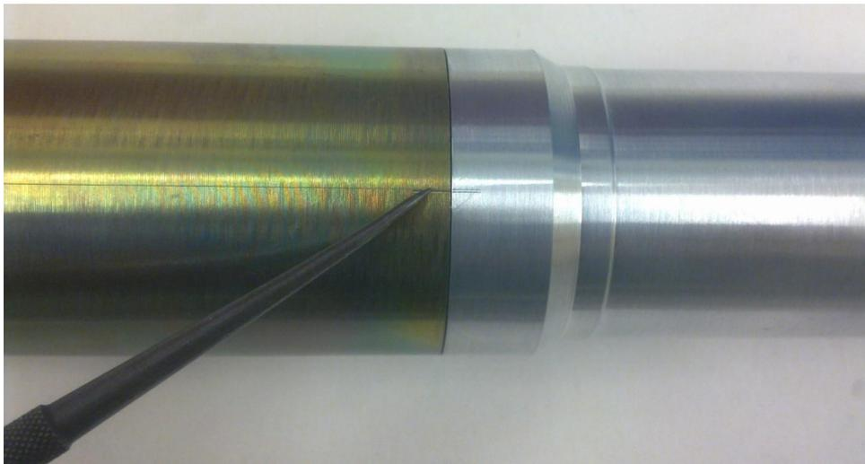
**Figure 4-1. The pointer indicates the score used to orientate the monitor to the neutron beam. The bead array is in this plane, so should be positioned perpendicular to the neutron beam direction.**
