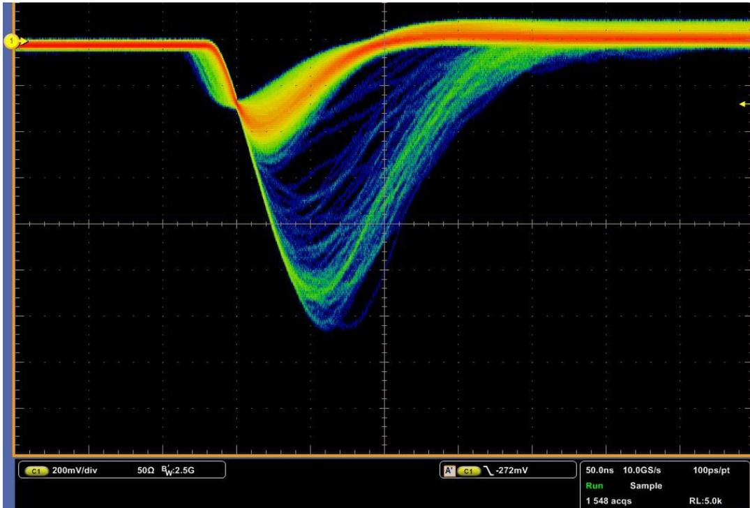
Figure 5-1. The Neutron Beam Monitor signal viewed using an oscilloscope connected to the ‘MON’ connection on the discriminator card. The monitor is being irradiated by an AmBe neutron source
