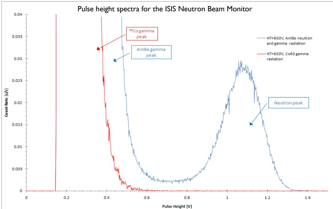
Figure 3-2. Pulse height spectra for the Neutron Beam Monitor DEMO I. The red data is for the gamma source  $^{60}\text{Co}$ . The blue data set is for the radiation from an AmBe source, which is a gamma and neutron mix. Note the data sets have been normalised arbitrarily for display purposes.
