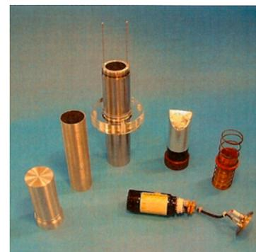
These monitors are used for data normalisation and in a diagnostic role to determine correct settings of beam line equipment including choppers, jaw settings and beam line scrappers. More than eighty ISIS Neutron Beam Monitors of this type are in use on ISIS. The majority of the ISIS neutron beam monitors are based on scintillation technology.
